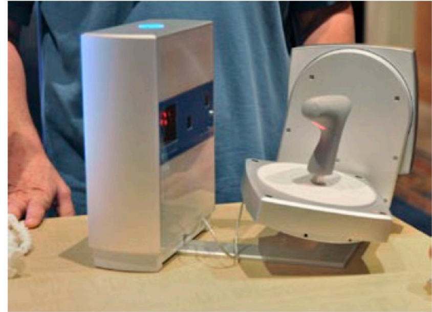
NextEngine Desktop 3d scanner with its Multidrive accessory, that allows non-contact 3d scanning.
